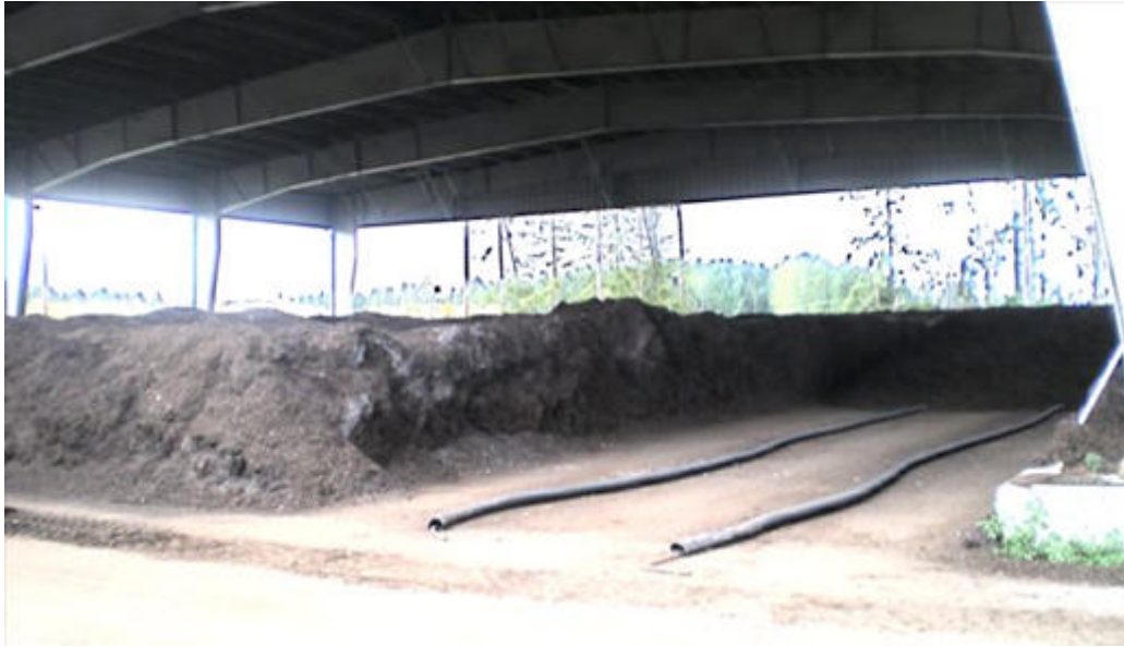
Secondary composting under cover, showing 'Big-O' aeration pipes, Bevan Road
